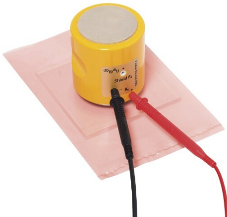
Sample application: Measurement with concentric ring probe
