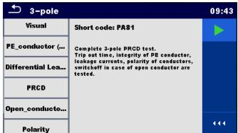
The combination of the different functions are built into several AUTO SEQUENCE®s which guide the user through complete and professional testing of P-RCD protected extension leads or portable switchgears. This functionality makes MI 3360 OmegaGT XA a leading tester in this application.
