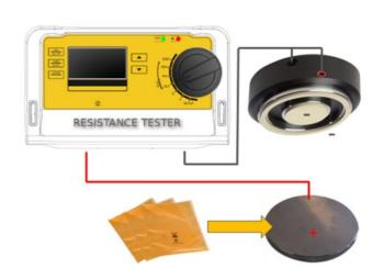
Surface resistance measurement R<sub>s</sub>
