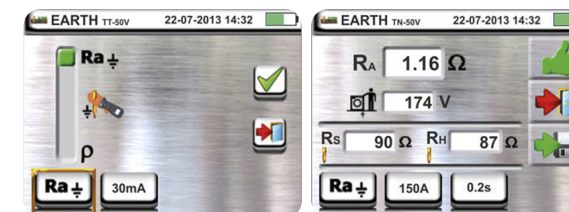
Earth resistance measurement by Volt-ampere method
