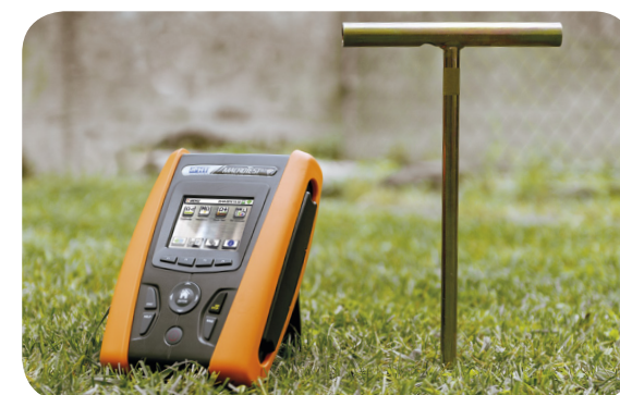
Earth resistance measurement by Volt-ampere method
