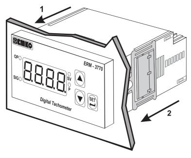
The unit is designed for panel mounting.
