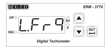
If the input frequency is lower than 0,07 Hz, then this screen will appear.
