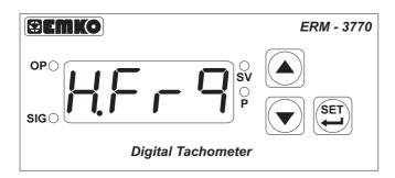
If the input frequency is higher than 10000 Hz, then this screen will appear.
